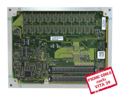
VITA-59 standard which specifies the mechanics to make COM Express modules suitable for operation in harsh environments.
