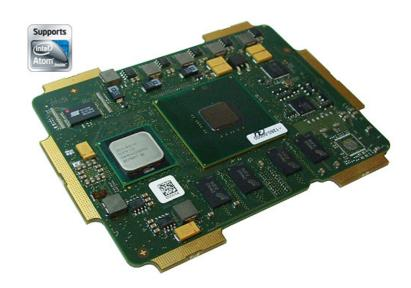
The XM1L is a Computer-On-Module of the ESMexpress® family. Together with an application-specific carrier board it forms a semi-custom solution for industrial, harsh, mobile and mission-critical environments.
