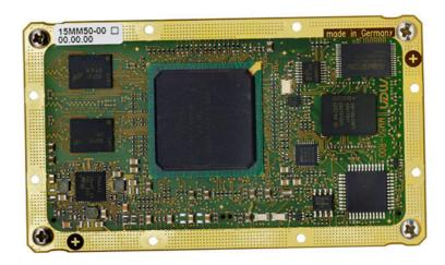
The MM50 is an ultra-small Computer-On-Module of the rugged ESMini™ family. Together with an application-specific carrier board it forms a semicustom solution for industrial, harsh, mobile and mission-critical environments.
