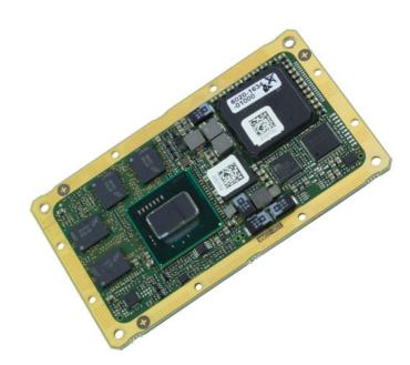
The MM2 is an ultra-small Computer-On-Module of the rugged ESMini<sup>™</sup> family. Together with an application-specific carrier board it forms a semicustom solution for industrial, harsh, mobile and mission-critical environments.
