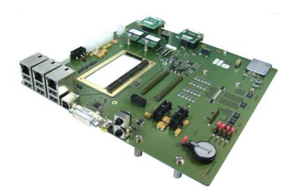
The XC4 is an evaluation and development platform that can be used together with any type of ESMini<sup>™</sup> module. It provides physical interfaces and connectors for nearly all of the modern serial standard I/Os routable from the ESMini<sup>™</sup> connectors to the carrier board. The XC4 comes with one ESMini<sup>™</sup> slot and two PCI Express® card slots. The functionality of all
