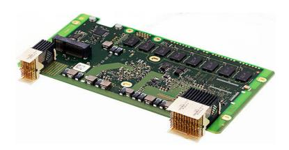
The SC24 is a maintenance-free single-board computer designed to serve as the heart of MEN's box and display computer systems for use in commercial vehicles, mobile machines, railway applications, avionics and industrial automation.
