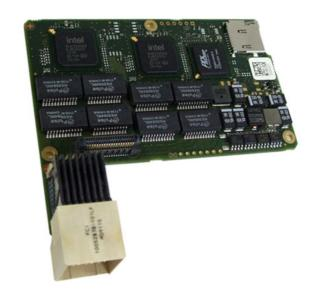
The GM2 is a mezzanine card which is plugged onto CompactPCI® Serial CPU boards to implement eight Ethernet interfaces on the backplane.
