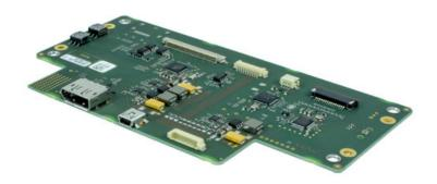
The adapter board also includes a temperature sensor and a brightness sensor to control the display and its backlight. Additionally a touch controller can be connected via USB. A key interface for connecting the display's external keys is also available on the AE63. The board operates within an input voltage range of 12 V to 24 V and is suitable for operating temperatures of -40 to 85°C.
