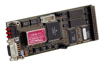
The M57 is a Profibus DP (Distributed Peripherals) interface. The M-Module is based on the ASPC 2 controller and the 16-MHz Motorola MC68331 CPU. It is an ideal interface solution for intelligent remote I/O applications via a very popular fieldbus standard. The ASPC 2 is an advanced Profibus controller allowing 127 stations with 254 SAPs (Service Access Points) each. It allows data transfer rates of up to 12 Mbaud on the M57.
