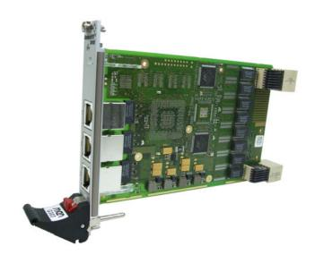
The G303 is an unmanaged 3U Ethernet switch implemented as a CompactPCI® Serial board. It occupies one peripheral slot, using a 4 HP front panel with 3 Gigabit Ethernet ports on RJ45 or M12 connectors. The G303 either features three Ethernet ports on the front and up to 13 Ethernet ports on the rear or alternatively all 16 Ethernet ports on the rear, which is the ideal solution for conduction cooling.
