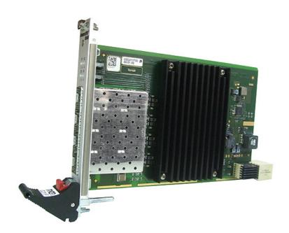
The G211F is a rugged 3U CompactPCI® Serial peripheral board. It offers the possibility to implement four optical fiber Ethernet interfaces. The board is equipped with a cage for connection of four SFP transceivers. The cage hosts the optical adapter. The cables are connected to the adapter module. MEN offers an optical transceiver with LC-Duplex connectors as an accessory.
