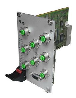
The F302 is a managed 3U Fast Ethernet switch module with a maximum of eight channels at the front panel (8 RJ45 or M12 connectors) plus one additional Ethernet channel that is led to the CompactPCI® J1 connector at the rear.
