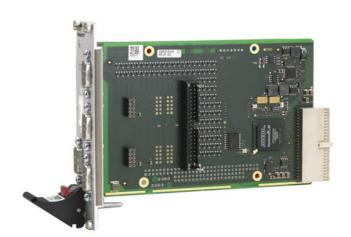
The F215 is a universal interface board based on 3U CompactPCI®. The physical layer can be realized individually for each channel by means of SA-Adapters™.
