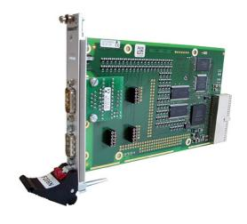
The Cyclone<sup>®</sup> FPGA acts as the main controller. It supports a 32-bit/33-MHz CompactPCI<sup>®</sup> bus, controls the SDRAM memory and has read/ write access to the Flash memory. The special FPGA-Flash structure provides initial programming using a boundary scan interface and later, with a configured FPGA, the device may be updated at any time with data from the CompactPCI<sup>®</sup> bus. The FPGA also controls four status LEDs and up to 79 user-defined I/O pins.
