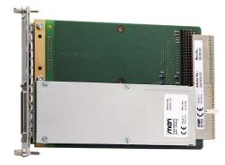
The F205 is a 3U M-Module carrier board for universal I/O on the CompactPCI<sup>®</sup> bus. It allows high flexibility in applications such as data acquisition or process control. The F205 is slightly higher than standard 3U format, providing enough space for two M-Modules while staying compatible with CompactPCI<sup>®</sup> housings
