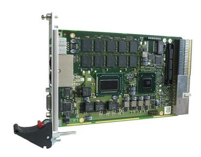
The F21P versatile 4HP/3U single-board computer is a continuation of MEN's proven range of Intel® CPU boards. It is equipped with the high-performance second generation Intel® Core™ i7 processor running at 2.1 GHz and offering the latest quad core processor architecture from Intel® with full 64-bit support. The CPU card delivers an excellent graphics performance and is designed especially for embedded systems which require high computing performance with low power consumption.
