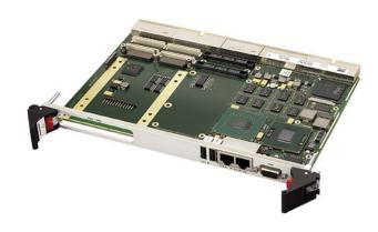
The D9 6U single-slot SBC supports a variety of Intel® Core™ Duo and Core 2 Duo processors from the highend 2.16 GHz T7400 to the low-voltage dual-core versions down to a selection of Celeron® M types. It is designed especially for embedded systems which require high computing and graphics performance and low power consumption.
