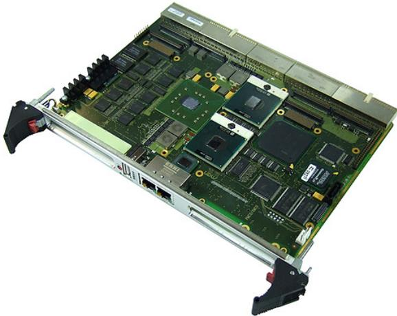
The D7 is equipped with two high-performance Intel® multi-core Xeon® processors, which consist of four CPU cores running at 1.66 GHz. The versatile 4 or 8HP/6U (single or double-slot, double-size Eurocard) CompactPCI® single-board computer is designed especially for embedded systems which require high computing performance. It comes with a tailored passive heat sink - forced air cooling is required inside the CompactPCI® system.
