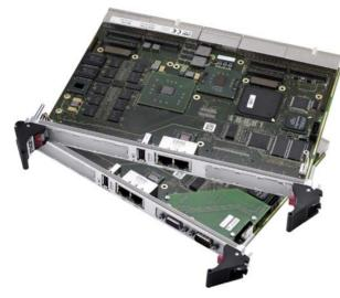
Equipped with the high-performance Intel® 2-GHz Pentium® M down to the 1-GHz ultra-low voltage Celeron® M processor, the D6 single-board computer is a versatile 4HP/6U (single-slot, double-size Eurocard) CompactPCI® Single-Board Computer, designed especially for embedded systems which require high computing performance. The SBC comes with a tailored passive heat sink within 4HP height - forced air cooling is required inside the CompactPCI® system.
