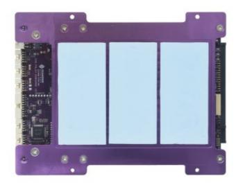
Bottom-mounted heat spreader / mounting plate with embedded thermal pads improves heat dissipation and simplifies assembly into enclosure
