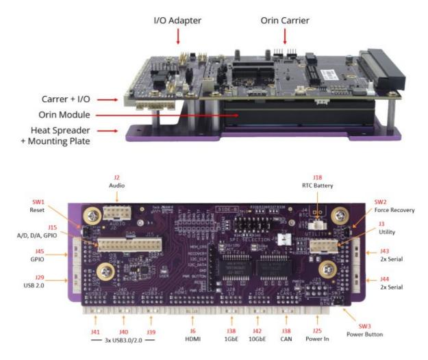
Osbourne-ER consists of two boards mated together: the main carrier board and the I/O adapter. The first diagram below shows the main carrier board, while the second diagram shows the I/O adapter. The two are joined via the block labeled "150-pin connector" to define the complete product architecture.
