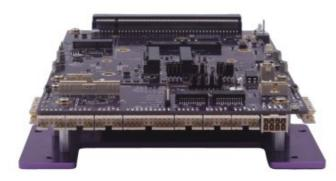
I/O adapter uses latching connectors for increased ruggedness
