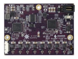
GMSL to CSI adapter module supports up to 8 GMSL cameras.
