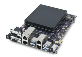
Osbourne carrier board with AGX Orin module and I/O connector board form the heart of JetBox-Osbourne.
