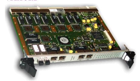
The 6760-6765 Series of switches are built on the latest generation of Gigabit switch engine technology managed by a PowerPC processor. The switch engine is based on a packet processor. The 6760-6765 Series supports full-wire speed L2 bridging with L2-L3 advanced traffic classification, filtering and prioritization providing traffic classification management needed for delay-sensitive or critical applications.
